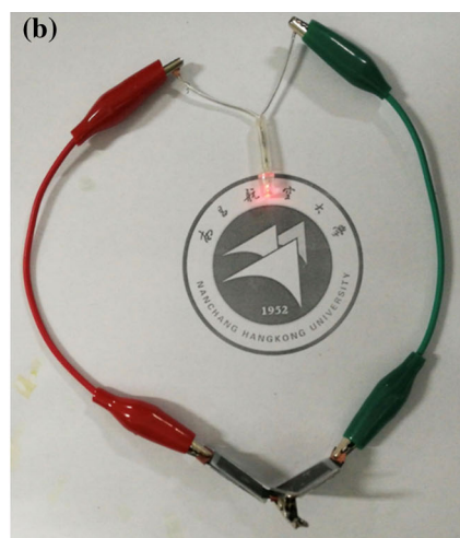
Figure 7 a Ragone plot of the MACC//Co(OH) 2 ASCs. b Two series-connected ASCs devices light a red LED.
